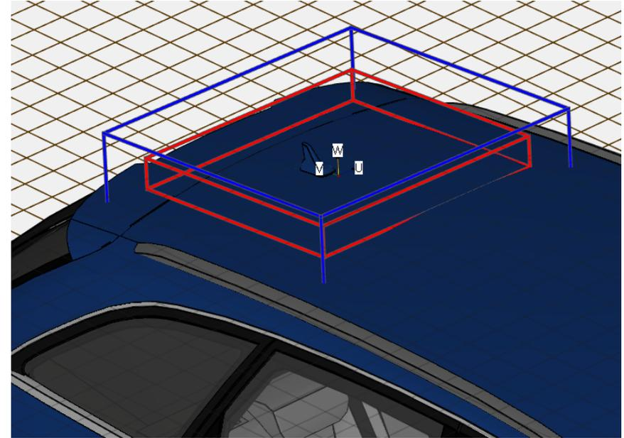
*Within the digital antenna twin field source placement, the u-direction corresponds to the x-direction in the measurement (v corresponds to y and w to z). As the sharkfin module should also be facing forward when using the antenna digital twin source, the u-direction must face forward. The upper right picture shows the u-direction pointing the left side of the car, so this can be achieved by a rotation around w axis.*
